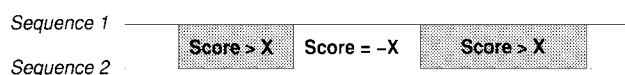
Fig. 1. Inclusion of an arbitrarily poor region in an alignment. If a region of score -X is sandwiched between two regions scoring more than X , the Smith–Waterman approach will join the three regions into a single alignment, regardless of how large X is.
